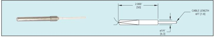
**The Series S Surface Mount Temperature Sensors** provide a cost effective and reliable solution for surface contact temperature measurement of conditioned water pipes, low pressure steam or refrigerant lines. The sensors are ideal for applications where immersion wells are not practical to install. Models are constructed with a 2 <sup>"</sup> (50 mm) 304 SS probe and a 6 ft (1.8 m) plenum rated cable. Nylon ties are included to secure the sensor to the pipe.
