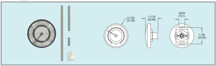
The Series BTP Pipe Mount Bimetal Surface Thermometers are designed to accurately measure the surface temperature of 3/4" to 6" pipe sizes. The BTP series includes three spring sizes to securely mount the pipe's surface. Pipe Mount thermometers are perfect for temporary installation and applications that require non-intrusive temperature measurement.
