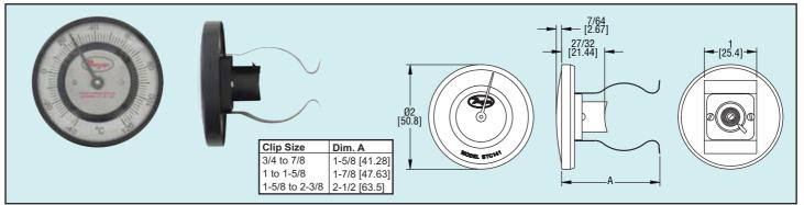
The Series STC Pipe-Mount Bimetal Surface Thermometers are designed to accurately measure the surface temperature of 3/4" to 2-3/8" pipe sizes. The STC series is available in three different clip sizes and feature a bimetal spiral spring sensing element that provides quick temperature readings. Pipe mount thermometers are perfect for temporary installations and applications that require non-intrusive temperature measurements.
