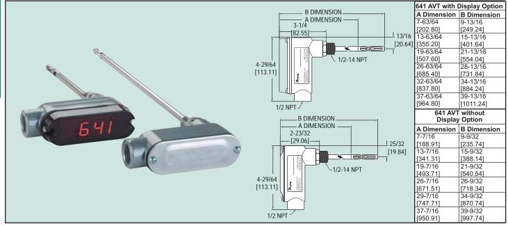
The new Series 641 Air Velocity Transmitter is the ideal instrument for monitoring air flow. This transmitter uses a heated mass flow sensor which allows for precise velocity measurements at various flow rates and temperatures. The 641's 16 field selectable ranges provides it the versatility to be selected for several air flow applications. The optional LED produces a complete, low-cost solution for local indication of air flow.
