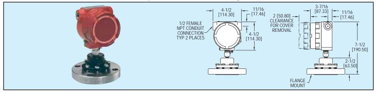
Series PLT Piezoresistive Level Transmitters provide reliable measurement and control of process levels by sensing the hydrostatic pressure in a tank. The loop-powered level transmitter delivers a 4 to 20 mA output signal proportional to hydrostatic pressure and specific gravity of the fluid for indicating, recording or control purposes. Easily accessible zero and span potentiometers make calibration in the field quick and simple. Units are equipped with EMI and reverse polarity protection.
