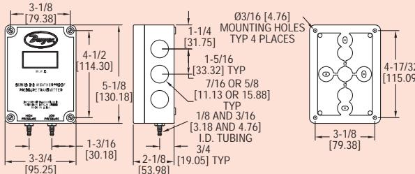
**Positive, negative and differential pressures can be measured** within a full span accuracy of  $\pm 0.25\%$  with the Series 616W Differential Pressure Transmitter. Units are enclosed in a polycarbonate case, rated NEMA 4X (IP66) and operate by sensing the pressure of air and compatible gases then sending a standard 4-20 mA output signal.
