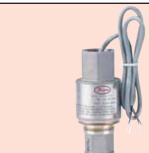
The Series 636 Pressure Transmitter is a low cost, fixed range, stainless steel transmitter with  $\pm 0.30\%$  accuracy. It is designed to continuously measure pressure for years in even the toughest environmental and media conditions. Select from 4 ranges to 0-300 psig (0-20 bar) with choice of 4-20 mA output (model 636) or 1-5 VDC output (model 636LP). Transmitters are explosion-proof, (FM approved) and meet NACE standards for offshore applications.
