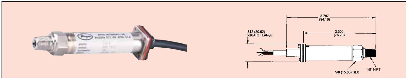
Series 638 Pressure Transmitters employ a polysilicon sensor for superior longterm stability and repeatability with  $\pm 0.5\%$  accuracy. They are FM approved intrinsically safe. Stainless steel NEMA 4X enclosure is ideal for corrosive media in hazardous environments. Output is 4-20 mA with 10-30 VDC power supply. NIST traceability with calibration certification is standard.
