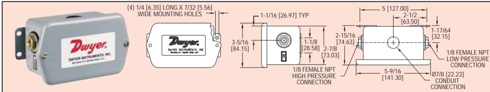
**Monitor differential pressure** in air/liquid flow systems, HVAC automation, pneumatic systems and process control with the Series 647 Wet/Wet Differential Pressure Transmitter. Units are temperature compensated and provide a 4 to 20 mA output signal which can be interfaced with chart recorders, data loggers and computerized monitoring and control systems.
