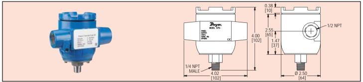
The Series 679 Pressure Transmitter is compatible with a wide range of gases and liquids, and is specially designed for weatherproof service (NEMA 4/IP56). The Model 679 can measure pressures with an accuracy of  $\pm .25\%$ . This model provides a 4-20 mA output and is field adjustable.
