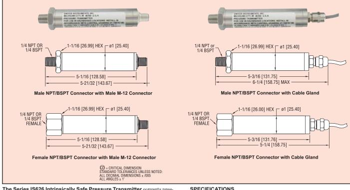
The Series IS626 Intrinsically Safe Pressure Transmitter converts pressure into a standard 4-20 mA output signal. The Series IS626 can be used to accurately measure compatible gases and liquids compatible with its 316/316L Stainless Steel wetted parts. Series IS626 full scale accuracy is 0.25%. Designed for industrial environments with a NEMA 4X (IP66) housing, this transmitter resists most effects of shock and vibration. Models are available with a 3 ' cable or M-12 4 pin connection.
