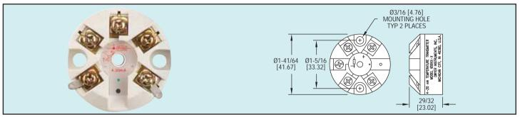
Series 659 Push-Button Temperature Transmitters accept thermocouple (J, K, T), RTD (Pt100 $\Omega$ ) or thermistor input and provide a linearized 4 to 20 mA output. The transmitter is quickly ranged and calibrated by using a single on-board switch. An LED provides visual indication of sensor fault and programming mode. Models feature reverse polarity protection. Thermocouple models are also galvanically isolated and cold junction compensated.
