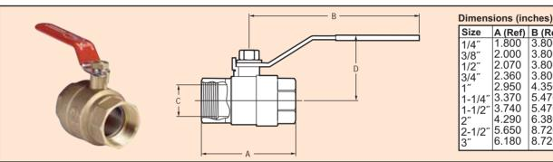
The Series BV2MB is an economical hand lever ball valve for commercial and general industrial use. The Series BV2MB is perfect as a manual shut off valve for hot and cold water systems. Valve body, body cap, and ball are made of quality brass. Seats and stem packing are constructed of TFE for long lasting service. Blowout-proof stem provides safety in the event of overpressure. Full port design allows for maximum Cv and minimal pressure drop.
