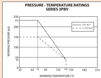
The Series 3PBV is ideal for mixing or diverting services in industrial, chemical, turf and irrigation, and pool and spa applications, as well as for use with potable water. The valve features a 3-seat design for efficient automation, reinforced TFE seats and EPDM seals for longer life, and an all PVC construction for heavyweight durability at a lightweight cost. Valves also come standard with field selectable NPT or socket process connections.
