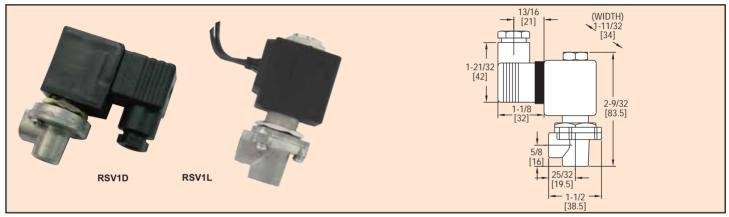
The Series RSV Pilot Solenoid Valve is used to operate the Series RDCV remote type diaphragm valve to air pulse clean filters in dust collectors. Consult factory for mounting of RSV valves with our DCT timer boards together in one enclosure all pre-wired.
