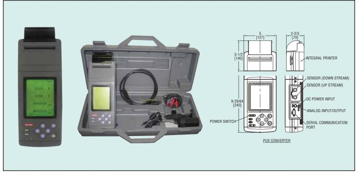
Series PUX Portable Ultrasonic Flowmeter Converters are paired with Series PSX2 sensors in order to utilize the transit-time difference for measuring flow rates in pipes from the outside. It is a compact and lightweight instrument incorporating the latest electronics and digital signal processing technologies, realizing high performance and easy operation. This portable unit is designed for 5 hours of continuous operation with its built-in battery, which only requires 3 hours to recharge.
