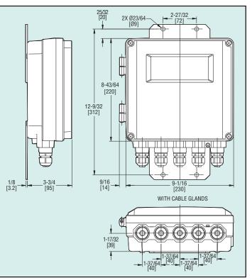
**Series UXF1 Ultrasonic Flowmeter Converters** are paired with Series SX1 or SX2 sensors in order to utilize the transit-time measuring method. Thanks to microprocessor based electronics, the flowmeter can easily be configured from the front keypad to specific applications. The flowmeter is suitable for liquid flow measurements for pipes from 1/2 inch to 19.5 feet diameter.
