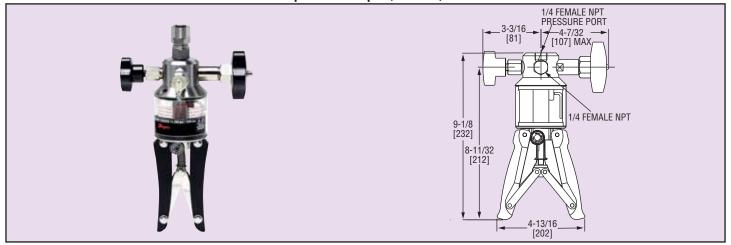
Generate pressures up to 10,000 psi (700 bar) with Model HHP-1 Hydraulic Hand Pump. Scissor action pump allows quick priming and pressure generation. Use in conjunction with an analog or digital pressure gage for a complete calibration system.
