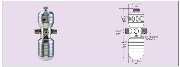
**Model HP Hand Pump** provides a dual source of pneumatic pressure and vacuum for verifying the calibration of pressure instrumentation. Pump can generate pressures up to 45 psig (3 bar) and vacuum to -27" Hg (-910 mbar). The compact pump is designed for portability and single hand operation.
