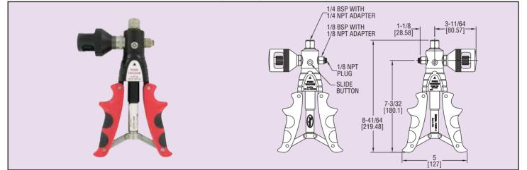
**The Series PCHP Pneumatic Hand Pump** comfortably sources pressure and vacuum to check calibration of gages, switches, transmitters, and recorders. The contoured cushion handles provide extra comfort while preventing the pump from sliding. The oversized check valve provides smooth operation throughout the output range. The dual o-rings on all pistons ensure zero leakage.
