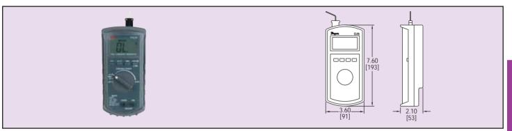
**Dual function** CA20 Thermocouple Calibrator can be used to source Type J thermocouple output values or measure Type J thermocouples. Quickly select output value using the rotary switch with coarse and fine adjustments. Model CA20 accepts up to two Type J thermocouples and features data hold and max functions. Measurements are displayed on a 3-1/2 digit backlit display. Units include a 4" (100 m) Type J bead wire temperature probe, calibration cable, 9V battery and instruction manual.
