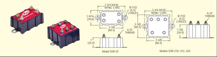
Series SSR Solid State Relays amplify the current handling capability of a variety of sensors for controlling higher power loads. The relays are compact, totally encapsulated and impervious to shock or vibration. Units feature SPST, normally open switch operation and can control loads up to 5A or 10A depending on model.
