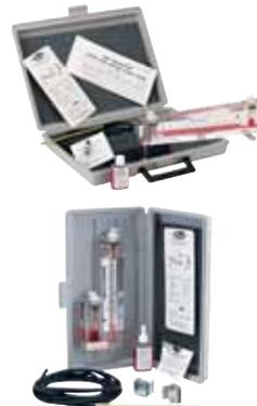
**100.5**, solid plastic portable gage with .10-0-1.0" w.c. range. Shown with carrying case and standard accessories.
