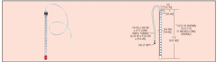
**Provide visual indication of pressure** with the Series 1213 Gas Pressure Manometer. Designed for use with natural gas, the manometer can also be used to monitor any compatible gases up to 15 inches of water column. Tap water is used as the sensing media and a magnetic clip provides temporary or permanent mounting. Economically priced and made of durable plastic for years of trouble-free service. Includes three feet of vinyl tubing and 1/8" nylon male NPT to barb fitting.
