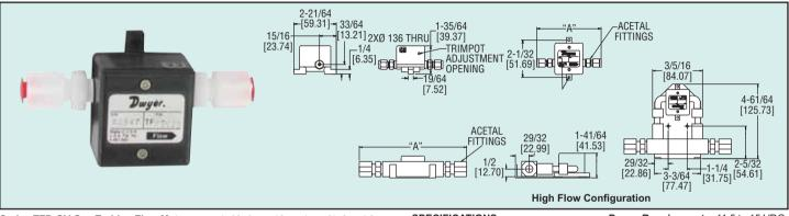
Series TFP-GV Gas Turbine Flow Meters are suitable for a wide variety of industrial, commercial, and laboratory flow applications. These meters utilize a turbine wheel and electro-optical detection to convert flow rates into a linear 0 to 5 VDC output signal for recording and data logging. Couple this unit with a Series FIV Flow Totalizer for a remote flow monitoring display. A power adapter or mating cable assembly is required for operation.
