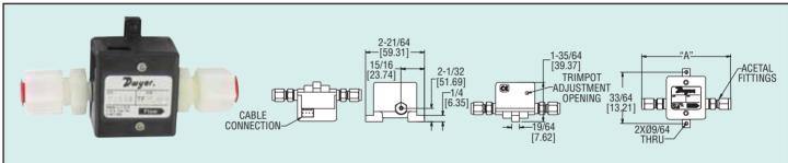
Series TFP-LP Liquid Turbine Flow Meters are suitable for a wide variety of industrial, commercial, and laboratory flow applications. These meters utilize a turbine wheel and electro-optical detection to convert flow rates into a linear 0 to 5 VDC output signal for recording and data logging. Couple this unit with a Series TM2 Flow Totalizer for a remote flow monitoring display. A power adapter or mating cable assembly is required for operation.
