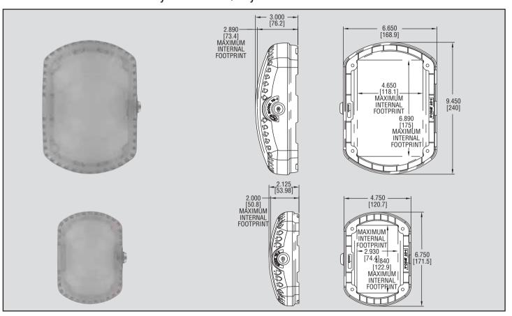
The Series TG Polycarbonate Thermostat Cover prevents physical damage and unauthorized adjustments of thermostats. Two sizes of covers are available to fit most common thermostats and transmitters. The low profile design with ventilation slits allows exceptional air flow in order to obtain accurate measurements. Each cover comes with two keys and mounting hardware for drywall and concrete walls. Model TG-1, Large Thermostat Cover Model TG-2, Small Thermostat Cover
