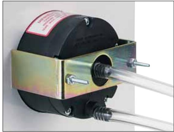
Mounting hardware is supplied with the MiniHelic® II gage for panel mounting through a single hole, 2-5/8" (67 mm) in diameter. Panel thickness up to 1/2" (13 mm) can be accommodated with the hardware supplied. If necessary, surface mounting of the gage can be accomplished by means of two 4-40 screws into the tapped mounting bracket stud holes in the rear of the gage. Surface mounting requires clearance holes in the panel for the two pressure taps.
