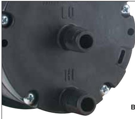
**A.** The standard Minihelic® II gage is supplied with two barbed pressure taps molded into the rear housing of the gage. These connections allow easy, fast connection to the gage using 3/16" I.D. rubber or plastic tubing.
