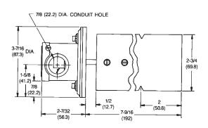
The Model 530 Air Flow Switch provides excellent sensitivity and reliability at a very reasonable price. Quality features include rugged die cast zinc body, stainless steel vane, silicone rubber gasket and SPDT snap switch. Unit is easily field adjustable from 400-1600 FPM. Mounting is fast and simple, requiring only two screws. Vane fits 6 in. or larger ducts. UL approved. To order, specify Dwyer Instruments, Inc. Model 530 Air Flow Switch.
