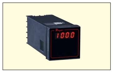
Low cost 1/16 DIN units provide 3-1/2 digit, 0.3" high LED readings from four field selectable input ranges. Includes integral power supply to operate 2-wire transmitters. Optional low/high SPST alarm relays can be set for direct or reverse action.
