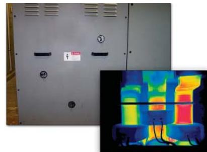
The SpyGlass lens attaches to the Mikron 7500, 7600 or 7800 cameras (also compatible with older models 7515, 7200, 7102) allowing the lightweight, high performance infrared camera to view entire electrical panels from just inches away.
