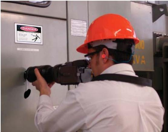
Raising the safety and convenience standard for thermal inspections, the SpyGlass Lens and ViewPort encourage frequent examinations of electrical switchgear because – with cabinet doors closed – no downtime is required to de-energize circuits for safety reasons.
