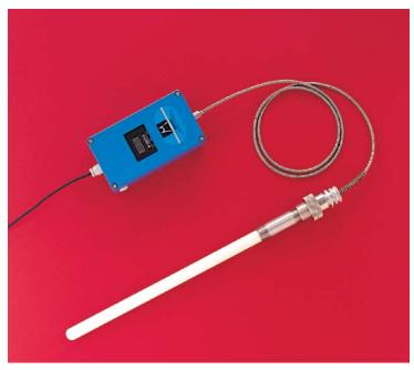
The M600 System is composed of a protective thermowell, infrared lens assembly enclosed in a stainless steel housing, fiber optic cable enclosed in a stainless steel sheath and a temperature transmitter enclosed in a water and dust proof housing.
