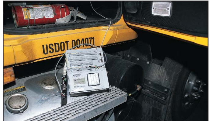
The SDM-CAN (left of CR5000) allows a vehicle's on-board diagnostic system to output standardized data streams that are synchronized with other measurements and stored in the CR5000.
