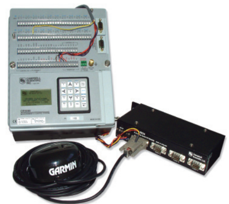
The sensor interfaces with the datalogger via the RJ45 to RS-232 Adapter and an SDM-SIO4 module. This interface option is compatible with our CR800, CR10X, CR1000, CR3000, CR5000, and CR9000X dataloggers.
