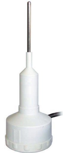
The 43347 probe connects to two differential channels and an excitation channel on the datalogger.
