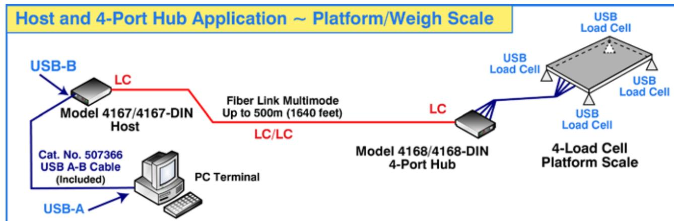
**USB A-B Cable (6 FT):** Included with Model 4167 / 4167-DIN is the cable ESL Cat. No. 507366. (USB Type A to USB Type B)
