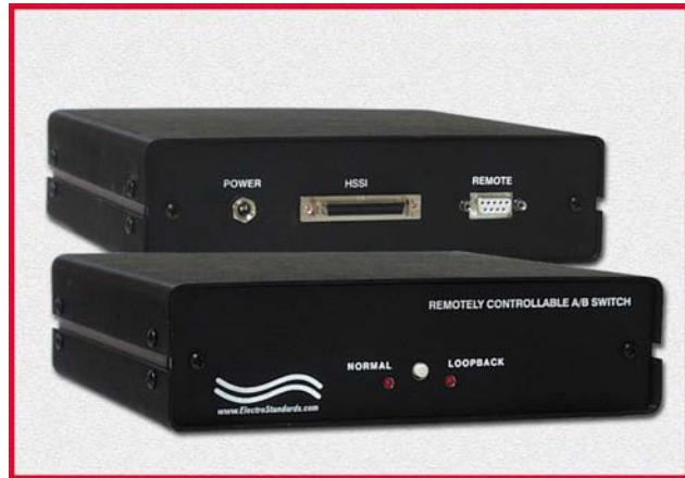
The Model 7432 Normal Loopback Switch is designed to Loopback key signals within a single HSSI port interface based on the presence or absence of the RTS signal on the DB9 port "REMOTE" (Automatic Mode), or based on the user depressing the front panel pushbutton switch. The HSSI interface is a 50-pin micro-D type connector. If the operator overrides the Automatic Mode, the user can alternate between Normal and Loopback positions regardless of the RTS signal on the DB9 port.
