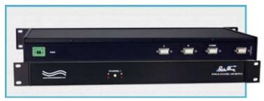
The switch may be controlled locally by manually operating the front panel pushbutton or remotely from the DB9/female serial interface Control port located on the rear of the unit. Switch position states may be attained locally via the front panel LED display or remotely using RS232 serial data commands.
