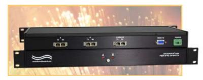
the unit. The DB9 Remote port provides contact closure control and also allows the user to monitor the switch position remotely through a set of dry contacts. The front panel LED display indicates the switch position and unit power status.
