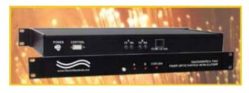
installs in a standard 19" equipment rack, and is 1U in rack height (1.75").
