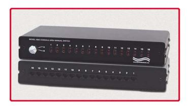
The Model 4855 is designed to provide remote switching and remote monitoring of up to sixteen Model 4875 Remotely Controllable KVM A/B Switches. A front panel two-position rotary switch provides the contact close transition or contact open transition signals required by the KVM switches for remote control operation. A/B status of all KVM switches connected to the Model 4855 are displayed via the front panel LED's.
