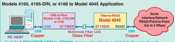
Isolated PC/HOST USB to RS422 communications serial interface/network.
