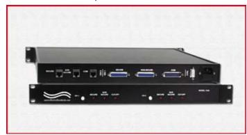
The switch may be controlled locally by manually operating the front panel pushbuttons or remotely from the DB9 Control port located on the rear of the unit using either contact closures or an RS232 command interface. The front panel LED displays indicate the respective switch position and unit power status.
