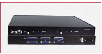
allow the user to set the switches to the "CUTOFF" position, which stops any and all data throughput for the switch. The switch may be controlled locally by manually operating the front panel pushbuttons or remotely from the DB9 Control port located on the rear of the unit using either contact closures or an RS232 command interface. The front panel LED displays indicate the respective switch position and unit power status.
