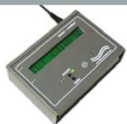
The Model 4337 has a multi-drop RS232/RS485 serial port that allows for connection of multiple units in a serial network configuration. This compact unit is ideally suited for in-situ transducer conditioning and distributed process measurements. It provides OEM users and system integrators with an affordable and complete strain gage-to-PC solution with intelligent display readout that is not found on competitive units.
