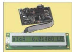
The Model 4327 features include nonvolatile memory for parameter and calibration storage, ability to select between 3 stored calibrations, automatic sensor identification using TEDS-Tag™ technology, solid state relay switches, multi-point and mV/V calibration, remote sense excitation, and 24-bit internal resolution with 16-bit analog output.
