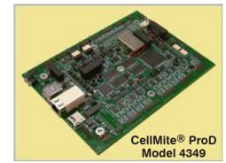
4349 perfect for recording important sensor data from transient applications such as pulsed power systems.
