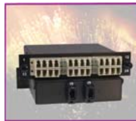
Model 6012 Two 12-Fiber MTP/MPO inputs break-out to 24 LC outputs (24 Simplex or 12 Duplex)
