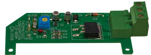
Miniature Temperature Control with Integral Sensor on Custom PC Board
