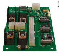
"H" Bridge Thermo-Electric **Heating-Cooling Control**
